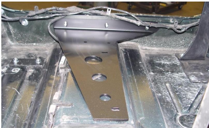
**STEP 3:** Reinstall seat bolts, and the remaining slider mounting bolts. Tighten all fasteners.
