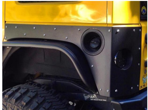
8. Place the driver's side Guardian™ Corner over the corner of the Jeep. The Guardian™ Corner will slip snugly over the fuel filler trim piece, helping to align the corner. Ensure that the distance between the top edge of the Guardian™ Corner and the top edge of the Jeep's tub is the same from front to back. When happy with the alignment securely clamp the Guardian™ Corner into place.
